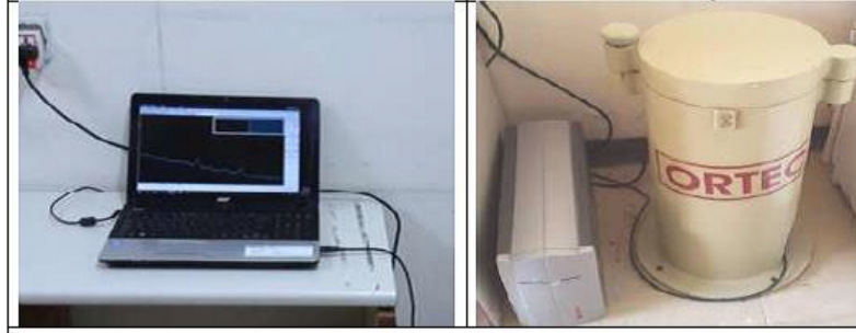
Figure 2: Experimental detection system setup with shielding and data acquisition components.
