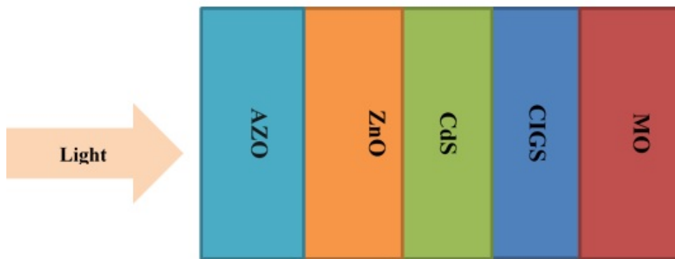
Figure 1: Solar Cell Structure AZO/ZnO/CdS/CIGS
