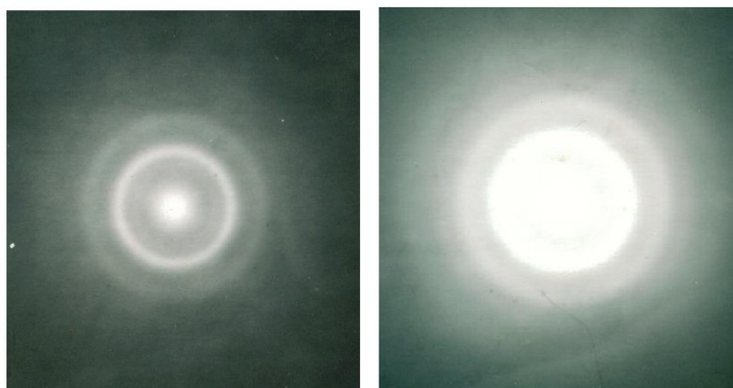
Figure 2: Electron diffraction pattern obtained from CuIn_5Se_8 (left) and CuGa_5Se_8 (right) amorphous thin films
