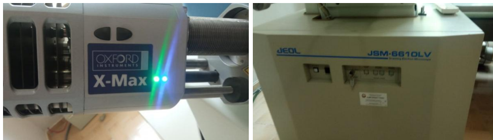
Figure 1: Scanning electron microscope (SEM) model JEOL JSM-6610LV-x-Max for research of HPPE+MWCNT composites.
