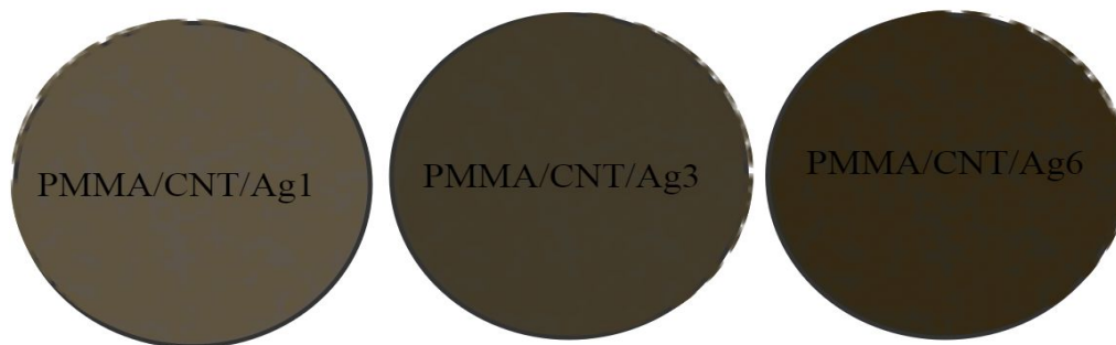
Fig.1: Digital photographic of the synthesized PMMA/CNT/Ag nanocomposites thin films, showing gradual color variation from gray to dark brown with increasing AgNPs concentration.
