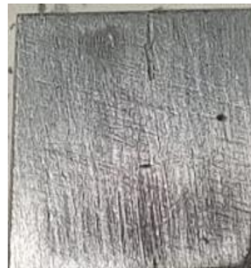
Figure 4. Photograph of a practical experiment on a steel sample using PF-1 corrosion inhibitor
