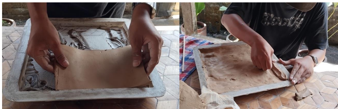
Figure 7. Process of Filling Soil in Molds Source: Researcher (2024)
